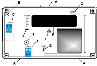
Figure 3 High power repeater internal components
