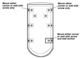
Figure 2 EN1260 mounting back plate
