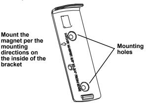
Figure 2 Mount the bracket
