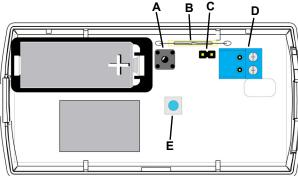
Figure 1 Door/window with reed switch internal components
