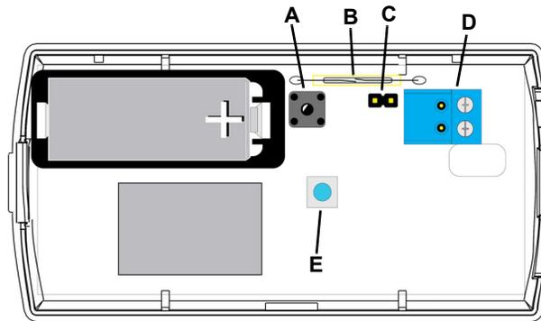
**Figure 1** Door/window with reed switch internal components
