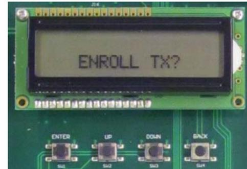
Press "Up" or "Down" to scroll thru the menu for other options or press "BACK" to exit programming mode. Screen will go blank.
